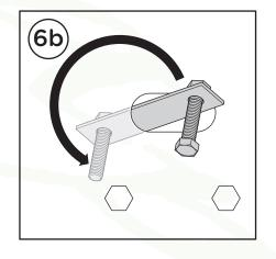
Pull the threaded side of the M8 Bolt + M8 Nut Plate through the bottom left hole.
