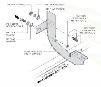
**9.** Fasten the top portion of the Passenger Side Rear Bracket to the bolt side of the M8 Bolt + M8 Nut Plate by using (1) M8 Flat Washer, (1) M8 Lock Washer and (1) M8 Hex Head Nut. Next, install the (1) M8 x 35MM Hex Head Bolt, (1) M8 Lock Washer and (1) M8 Flat Washer to the nut side of the M8 Bolt + M8 Nut Plate.
