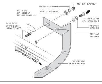
8. Fasten the top portion of the Driver Side Center Bracket to the bolt side of the M8 Bolt + M8 Nut Plate by using (1) M8 Flat Washer, (1) M8 Lock Washer and (1) M8 Hex Head Nut. Next, install the (1) M8 x 35MM Hex Head Bolt, (1) M8 Lock Washer and (1) M8 Flat Washer to the nut side of the M8 Bolt + M8 Nut Plate.
