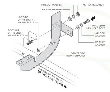
**9.** Fasten the top portion of the Driver Side Rear Bracket to the bolt side of the M8 Bolt + M8 Nut Plate by using (1) M8 Flat Washer, (1) M8 Lock Washer and (1) M8 Hex Head Nut. Next, install the (1) M8 x 35MM Hex Head Bolt, (1) M8 Lock Washer and (1) M8 Flat Washer to the nut side of the M8 Bolt + M8 Nut Plate.
