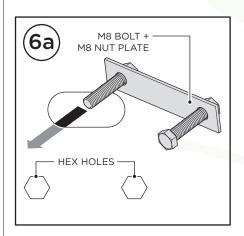
Rotate the threaded side of the M8 Bolt + M8 Nut Plate to the bottom left hole.
