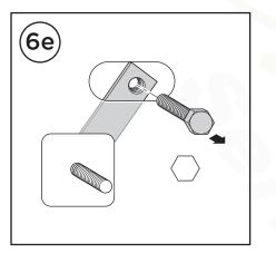
The M8 Nut Plate will now be able to rotate down to the hole in the rocker panel, allowing for bracket installation.
