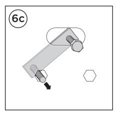
Install Plastic Retainer to ensure you do not drop the M8 Bolt + M8 Nute Plate into the rocker panel.
