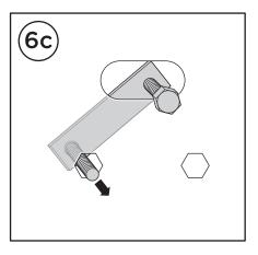
Install Plastic Retainer to ensure you do not drop the M8 Bolt + M8 Nute Plate into the rocker panel.
