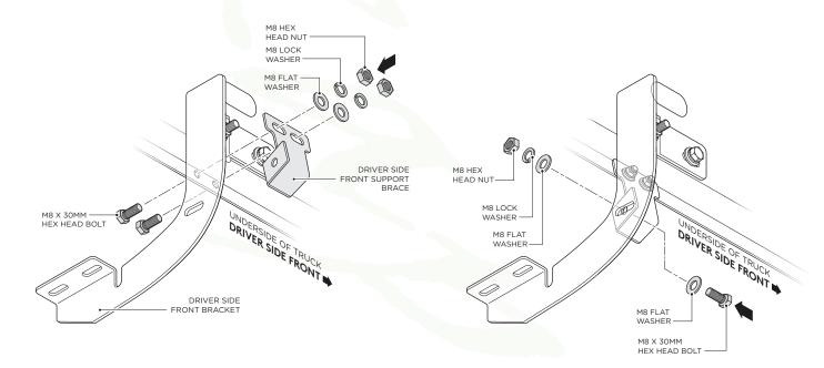
11. Fasten the top of the Driver Side Center Support Brace to the rocker panel using (2) M8 x 30MM Hex Head Bolts, (2) M8 Flat Washers, (2) M8 Lock Washers and (2) M8 Hex Head Nuts. Then, fasten the bottom of the Driver Side Center Support Brace to the Driver Side Center Bracket using (1) M8 x 30MM Hex Head Bolt (2) M8 Flat Washers, (1) M8 Lock Washer and (1) M8 Hex Head Nut.
