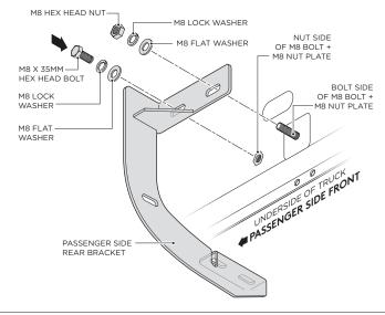
8. Fasten the top portion of the Passenger Side Center Bracket to the bolt side of the M8 Bolt + M8 Nut Plate by using (1) M8 Flat Washer, (1) M8 Lock Washer and (1) M8 Hex Head Nut. Next, install the (1) M8 x 35MM Hex Head Bolt, (1) M8 Lock Washer and (1) M8 Flat Washer to the nut side of the M8 Bolt + M8 Nut Plate.
