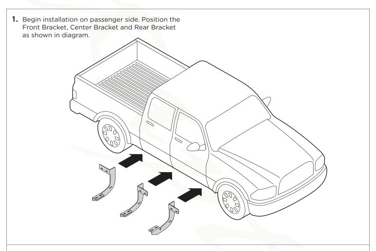
2. Passenger Side Front Bracket cradle (2a) will face to the rear of the truck. Passenger Side Center (2b) and Rear Bracket cradles (2c) will face toward the front of the truck.
