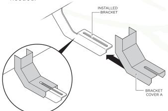
2. If trimming is necessary, carefully trim the Bracket Cover using scissors or a knife until you reach your desired look and fit (2a). Once this is complete, place the Bracket Cover A onto the installed bracket (2b).
