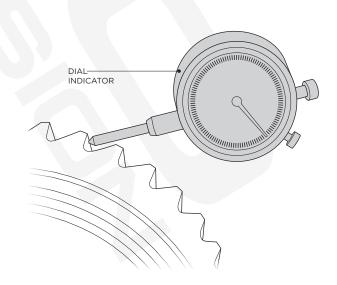
**25.** Adjust the thickness of the carrier shims to get the desired amount of backlash. The total carrier shim thickness should remain the same as the original shims. Whatever you take from one side, you need to add to the other side.
