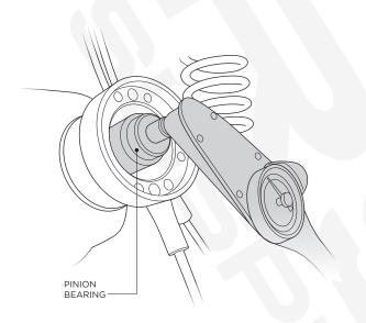
**16.** Carefully inspect all the bearings for any sign of abnormal wear. The bearings may be reused if this is a low mileage gear swap and if the bearings are in good condition.
