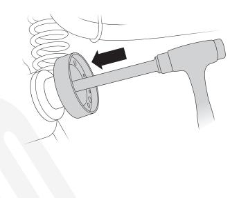
**17.** Using a 13/16" socket, remove the ring gear bolts. The ring gear should have a light press fit on the carrier. Thread a few of the bolts in the ring and tap the bolts so you can remove the ring gear. Be careful to not let the ring gear fall on the coil or wires for the locker.
