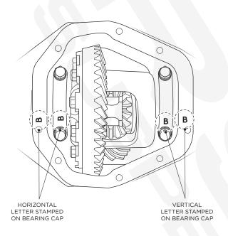
**12.** Remove the differential carrier assembly. Keep track of which side the carrier bearing races and shims came from. The bearing races must be installed on the side they were originally located.
