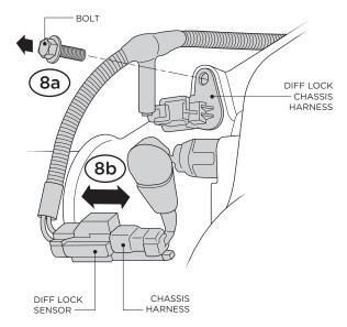
**9.** Using an 8mm socket, remove the diff lock bulkhead connector. Pull the connector from the housing and disconnect the locker coil wires from the bulkhead connector.
