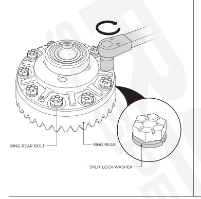
**20.** Clean the threaded holes in the ring gear and ring gear bolts with brake or carb cleaner. Early JK's used 7/16" ring gear bolts and the later JK's use 1/2" ring gear bolts. The ring is tapped for both.
