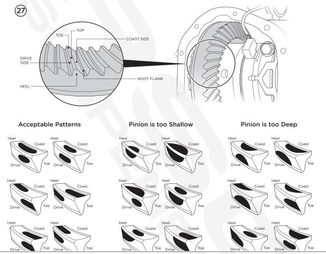
**26.** Once you have the backlash in spec, use the gear marking compound to check the gear mesh pattern. Paint about four (4) teeth on both the coast side and the drive side.
