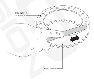
**18.** Carefully clean the ring mounting surface of the carrier and new ring gear.
