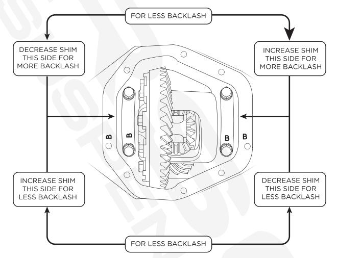
**29.** Once you have the backlash in spec, use the gear marking compound to check the gear mesh pattern. Paint about four (4) teeth on both the coast side and the drive side.
