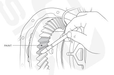
**30.** Next, you must read the gear mesh contact pattern.
