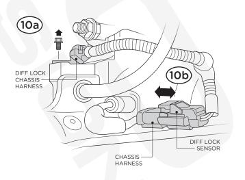
**11.** Using an 8mm socket, remove the diff lock bulkhead connector. Pull the connector from the housing and disconnect the locker coil wires from the bulkhead connector.
