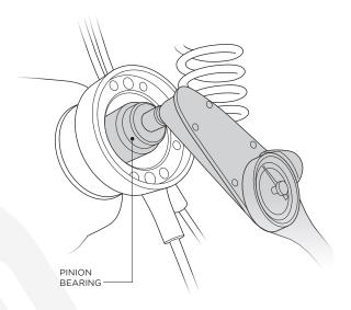
**18.** Carefully inspect all the bearings for any sign of abnormal wear. The bearings may be reused if this is a low mileage gear swap and if the bearings are in good condition.
