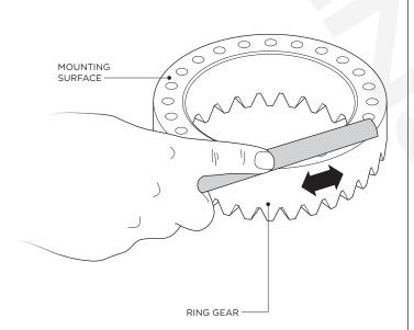
**20.** Carefully clean the ring mounting surface of the carrier and new ring gear.
