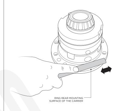
**22.** Clean the threaded holes in the ring gear and ring gear bolts with brake or carb cleaner. Place a measure of thread locker onto the first few threads of each ring gear bolt.
