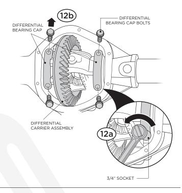
**14.** Remove the differential carrier assembly. Keep track of which side the carrier bearing races and shims came from. The bearing races must be installed on the side they were originally located.
