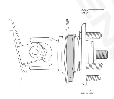
**5.** Remove the three (3) unit bearing bolts (two (2) from the inside of the knuckle) using a 13mm socket.
