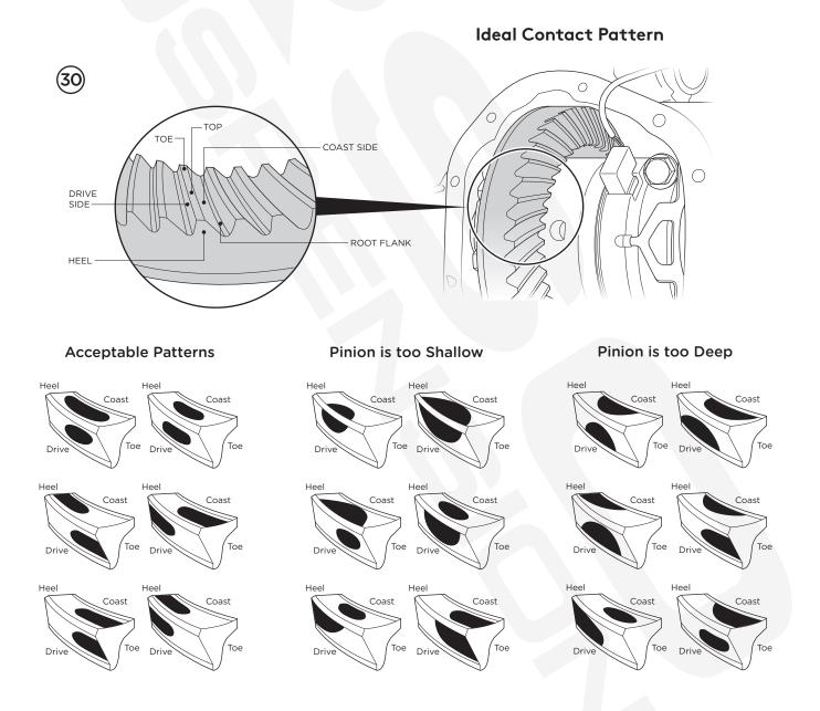
**31.** Once you have an acceptable contact pattern and backlash measurement, you may begin final gear assembly. Remove the carrier and pinion.
