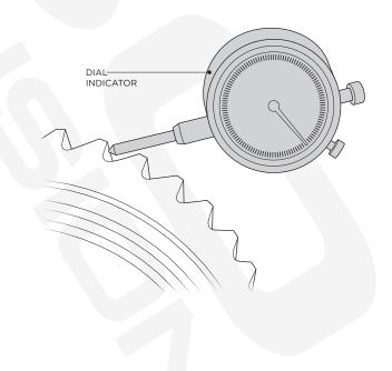
**28.** Adjust the thickness of the carrier shims to get the desired amount of backlash. The total carrier shim thickness should remain the same as the original shims. Whatever you take from one side, you need to add to the other side.
