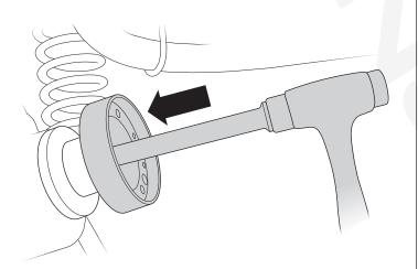
**16.** Use an in-Ib dial or beam type torque wrench to measure the pinion bearing torque to rotate. The torque to rotate should be in the 10-20 in-Ib range. Record this number in the diff set-up sheet for future installation if you are using the original pinion bearings.
