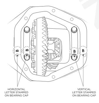
**12.** Using a 3/4" socket (12a), loosen and remove four (4) differential bearing cap bolts (12b) to remove the two (2) differential bearing caps.
